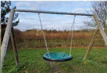
Finding: Swings of this design should have a secondary Action: Monitor use and check the joint and fixing security safety mechanism fitted to prevent collapse of the seat in the regularly event of a joint failure to comply with BS EN 1176 Part 2, however this swing was installed prior to the standards being updated in 2018 and the manufacturer has confirmed
