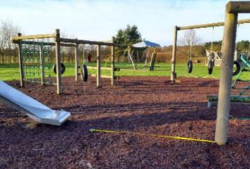
**Finding:** The impact area of the climbing frame overlaps the **Action:** Monitor - No remedial work recommended freespace of the slide in contravention of BS EN 1176
