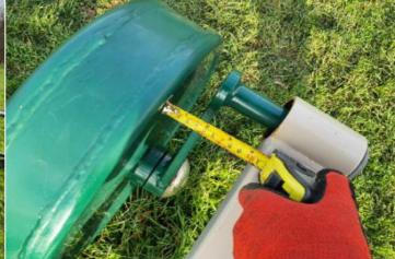
**Finding:** The distance between the crank and frame is between 8 and 60mm creating a potential crush/shear point in contravention of the requirements of BS EN 16630
