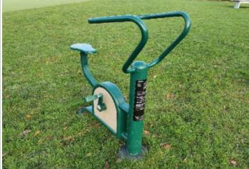
Finding: There are gaps between 8 and 60mm creating a potential crush/shear point in contravention of the requirements of BS EN 16630
